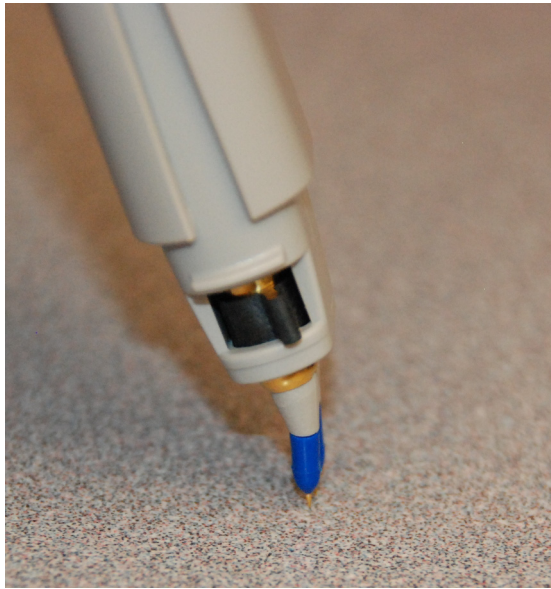
Figure 28 Proper Vertical Orientation of the Blue Tips
