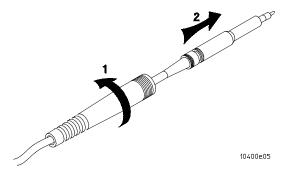
The cable strain relief may be unscrewed from the probe and slid back on the cable when using two or more probes in close proximity. When using the probe without the browser or retractable hook tip, the barrel insulator (supplied accessory) should be used to cover the tip ground shield to prevent the hazard of shorting when probing the circuit. The barrel insulator, may be unscrewed and removed to accommodate tight probing situations.
