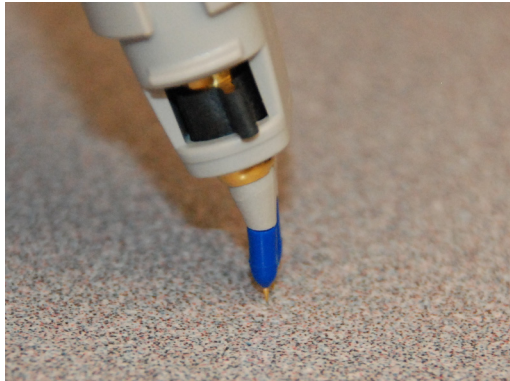
Figure 56 Proper Vertical Orientation of the Blue Tips
