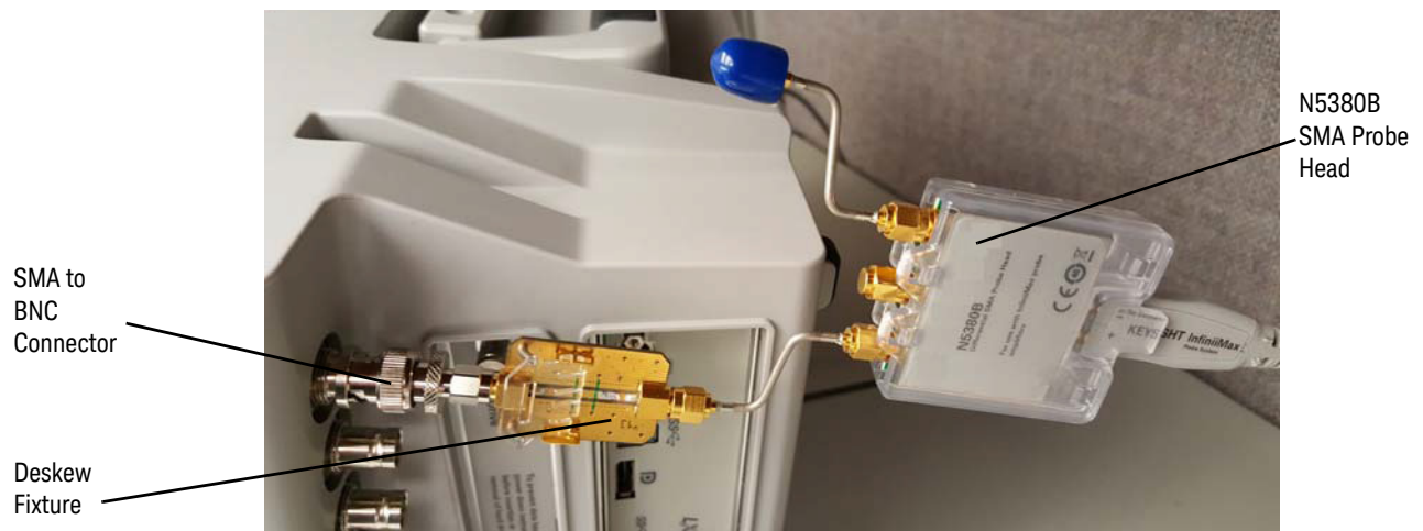
Figure 113 Connecting the SMA Probe Head and Deskew Fixture
