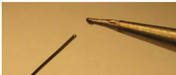
Figure 67 Small Amount of Solder Added to Soldering Iron Tip
