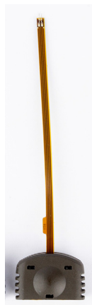
Discoloration after usage under high temperatures
