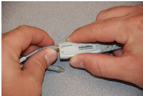
Figure 4 Properly Pulling the Probe Head Straight Out
