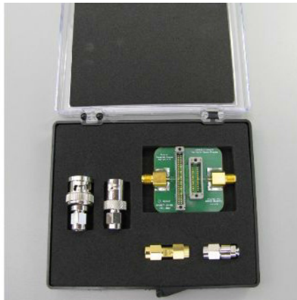
Figure 114 N2887-60002 Calibration/Deskew kit
