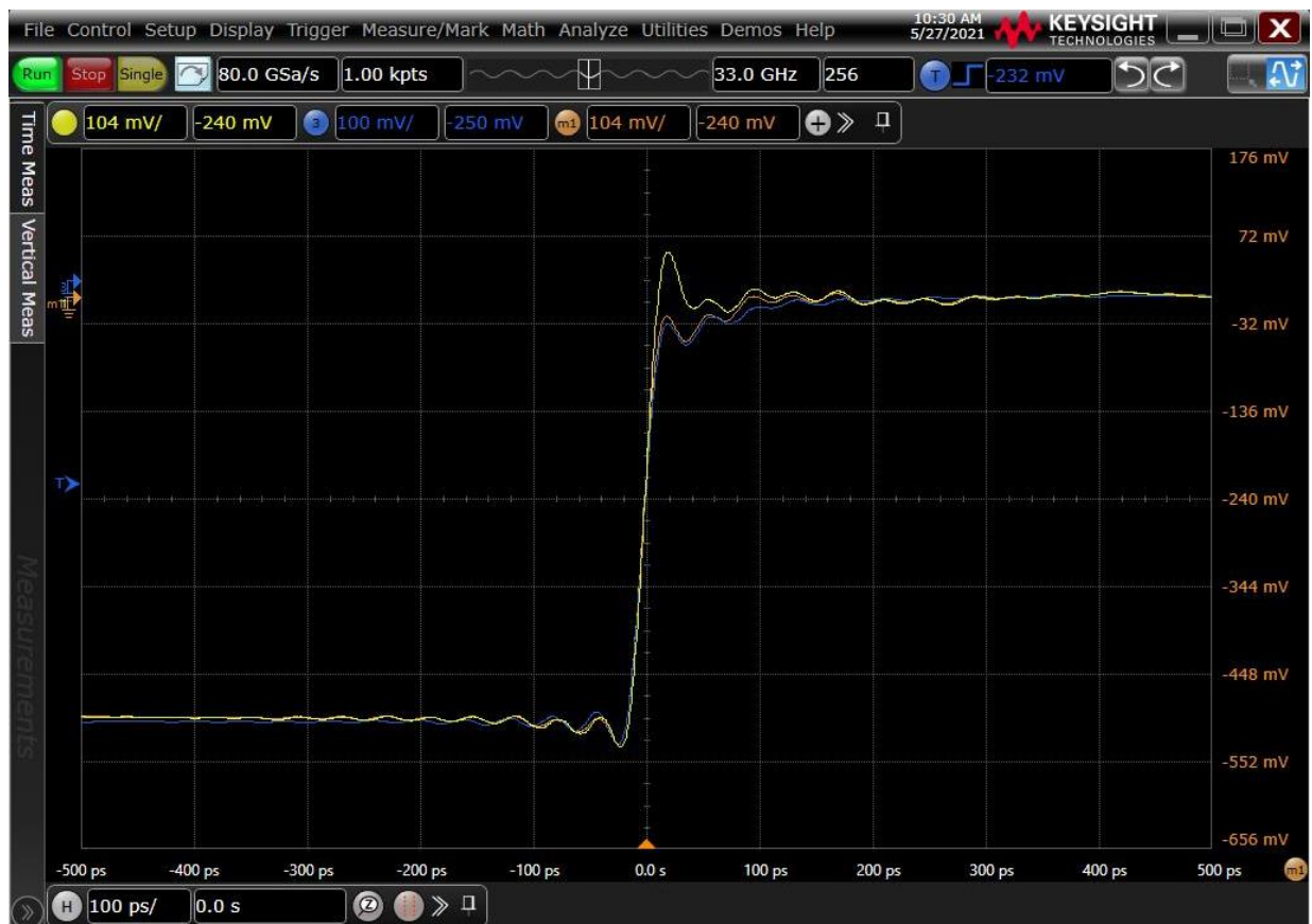
Figure 2. Visual depiction of the difference between signal ( V_{in} - blue trace), True View ( V_{out}/V_{in} - brown trace), and Source Estimate ( V_{out}/V_{source} - yellow trace).
