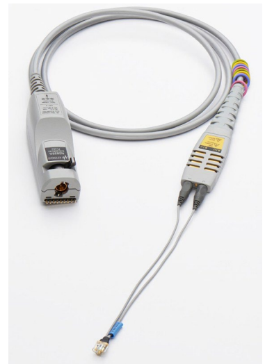
N2830A InfiniiMax III+ amp with QuickTiphead
