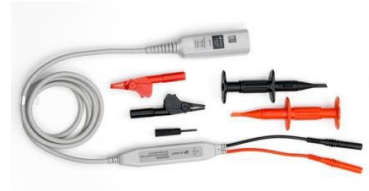
N2818A 200-MHz, 20-V differential probe
