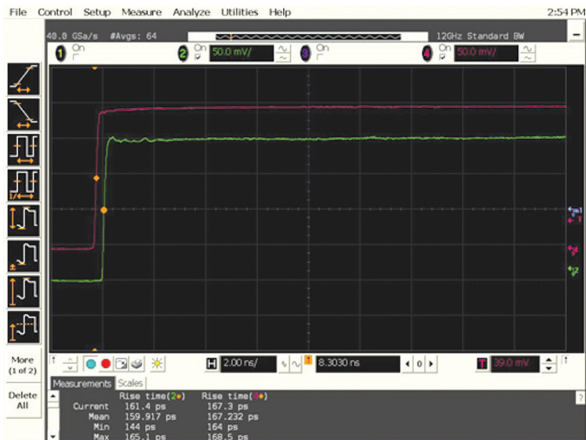
Figure 4 Time domain differential probe response, purple = input of the probe, green = probe output, using Keysight 1169A InfiniiMax probe and DS081304B 13 GHz oscilloscope
