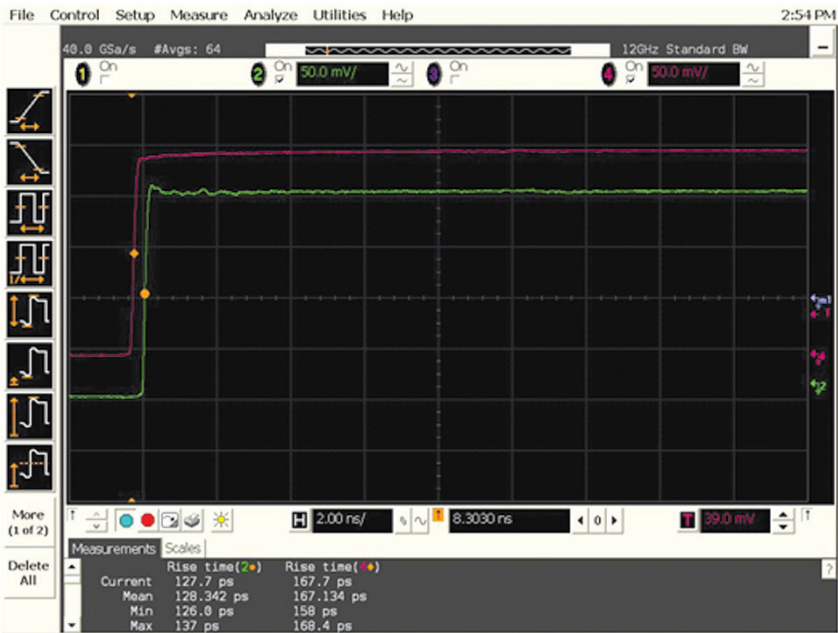
Figure 5 Time domain single-ended probe response, purple = input of the probe, green = probe output, using Keysight 1169A InfiniiMax probe and DS081304B 13 GHz oscilloscope
