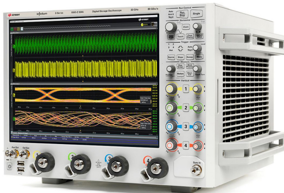
Figure 7. The N7024A 6GHz Power Rail probe is compatible with the V-Series and Z-Series (shown) oscilloscopes. Because these oscilloscopes have the AutoProbe II interface they require the N5442A Precision BNC adapter to be able to use the N7024A.
