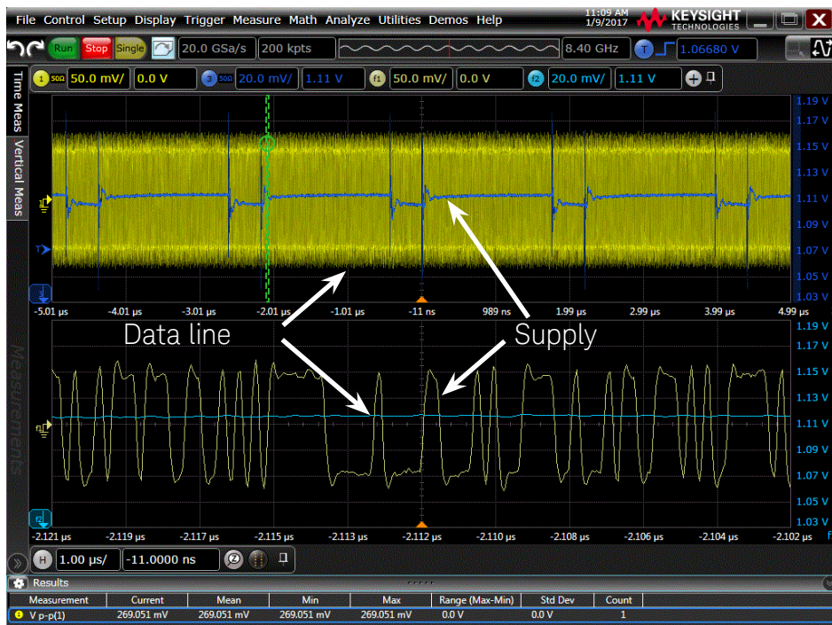
Figure 23. FPGA DC supply and the serial data captured by the S-Series oscilloscope.
