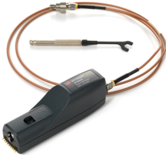
Figure 21. The N7024A with the included 1250-4403 rotating adapter attached to the main cable. The wrench shown is included with the N7024A and is for the removal of the rotating adapter
