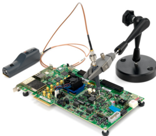
Figure 20. Example showing the N7032A or N7033A browsers in use, being held in place by the Keysight N2787A 3D probe positioner
