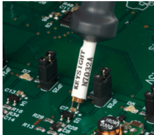
Figure 18. Close up view of the N7032A 4GHz power rail probe browser probing a small capacitor package on the power distribution network
