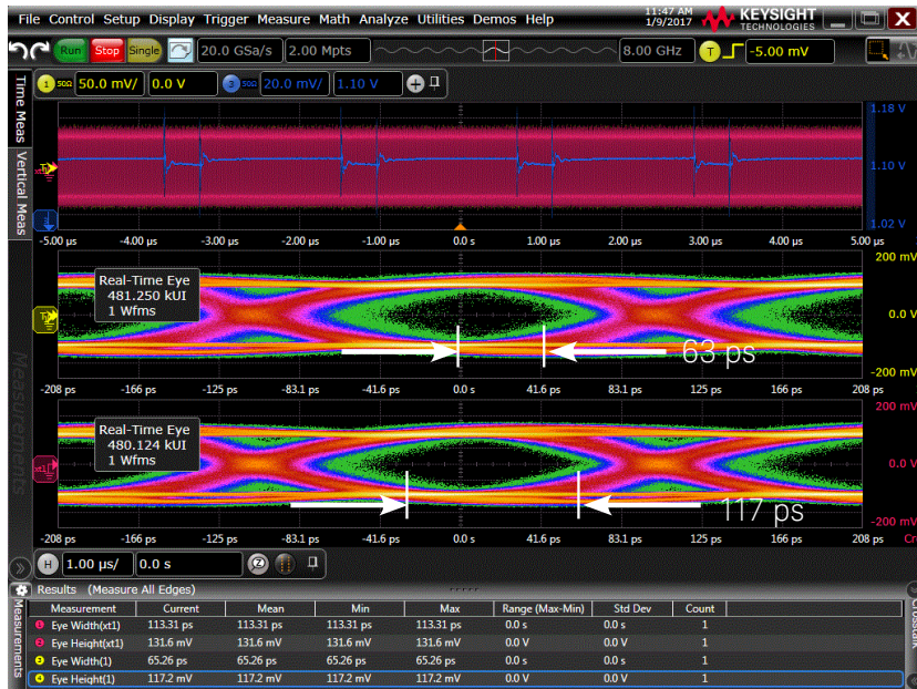
Figure 26. Results from the N8846A PI analysis application showing the eye diagram of the FPGA serial data before and after the effects of the DC supply noise are removed. Notice that the results are nearly identical to the previous results where the supply was physically change to reduce noise.
