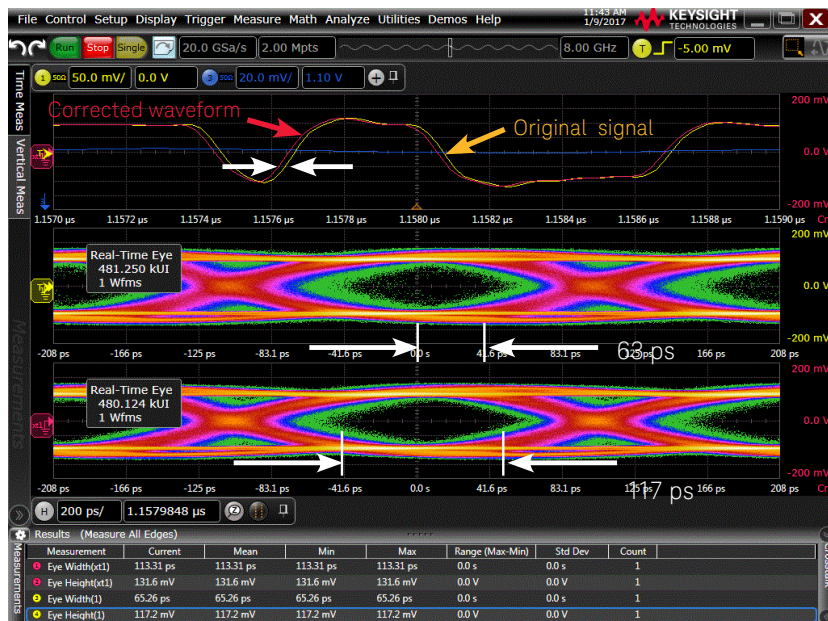
Figure 27. Expanded timebase view of the FPGA serial data with and without the effects of the DC supply noise.
