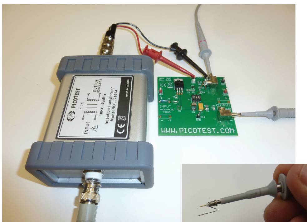
Figure 3: Probing the DC-to-DC converter using two channels of the oscilloscope.
