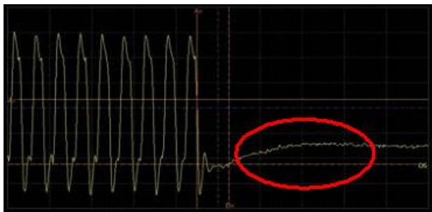
Figure 7. The eMMC data strobe line measured with a Keysight InfiniiMax probe with RCRC architecture
