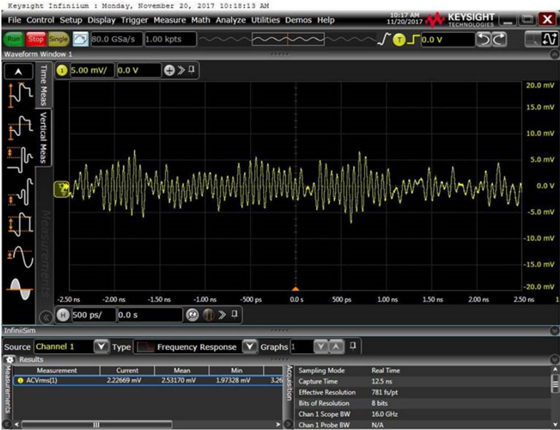
Figure 8 - The noise is at 2.5mVrms at 16 GHz, up 2x from 12 GHz and is “bursty” and “sine wavy”.
