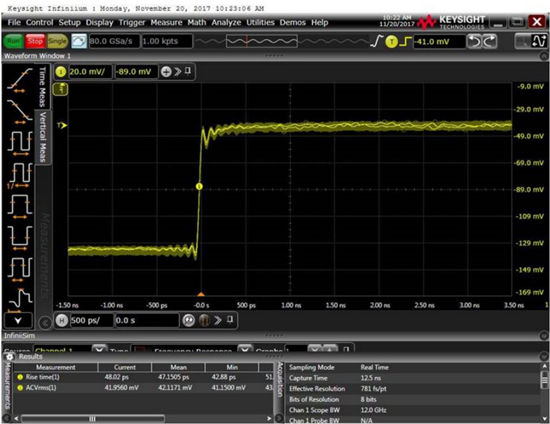
Figure 9 - At 12 GHz bandwidth, the rise time at 10-90% is 47.1 psec.
