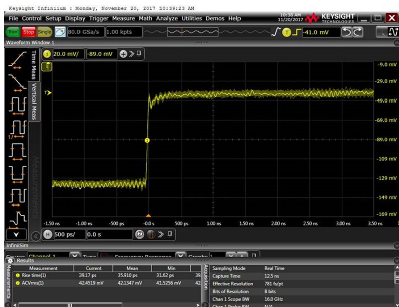
Figure 11 - At 16 GHz, the bursty and sine wave nature is obvious in the base and top so the bandwidth boosting is not very realistic at this bandwidth.
