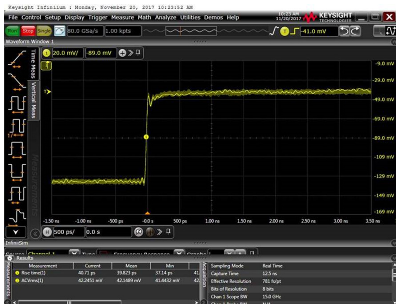
Figure 10 - At 15 GHz, the rise time gets faster at 39.8 psec.
