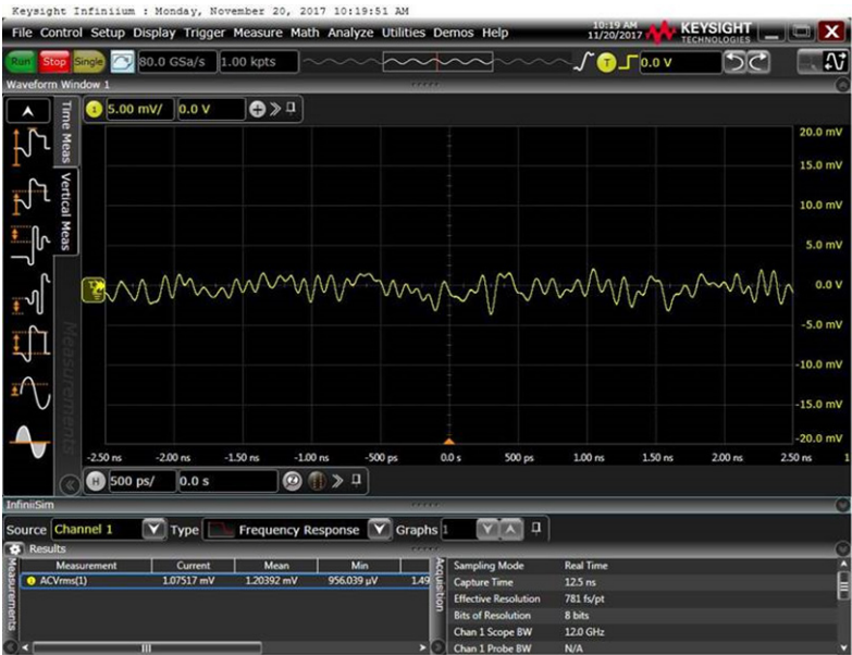
Figure 6 - The rms noise at 12 GHz is 1.2mVrms.
