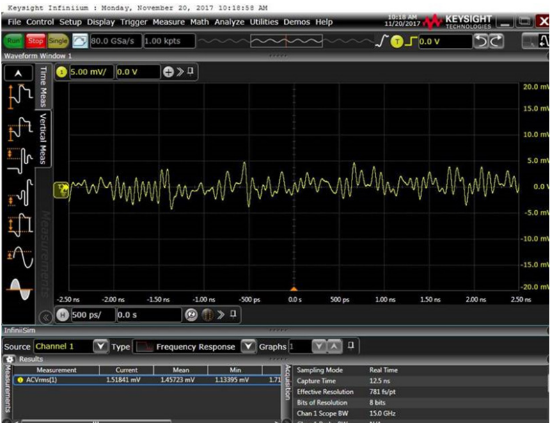
Figure 7 - The noise has gone up from 1.2mVrms to 1.46mVrms – up 21%, as the bandwidth is boosted to 15 GHz.
