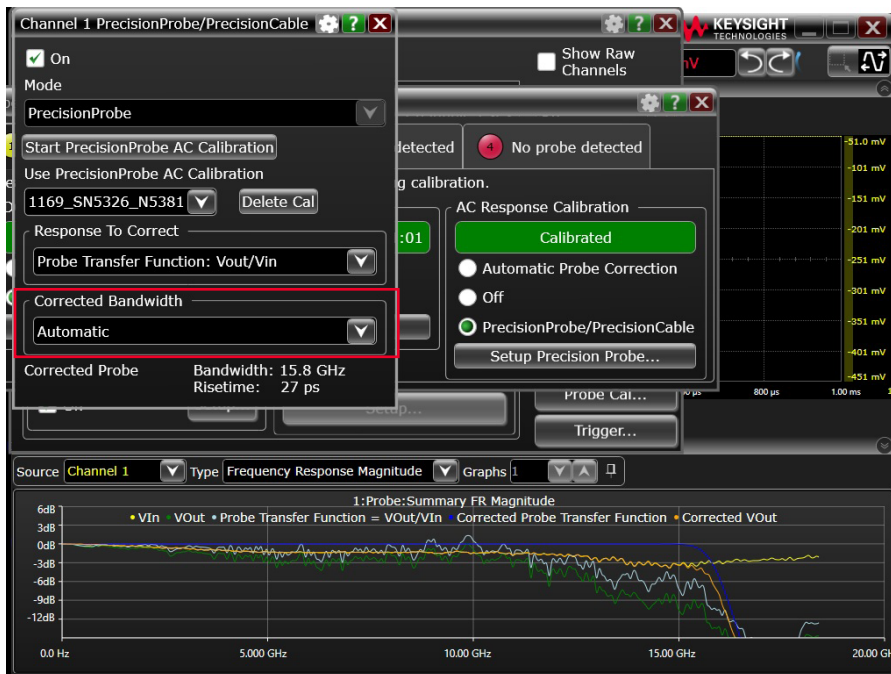
Figure 5 - The Corrected Bandwidth is set to Automatic and the PrecisionProbe calibration has made the bandwidth of the probe 15.8 GHz.
