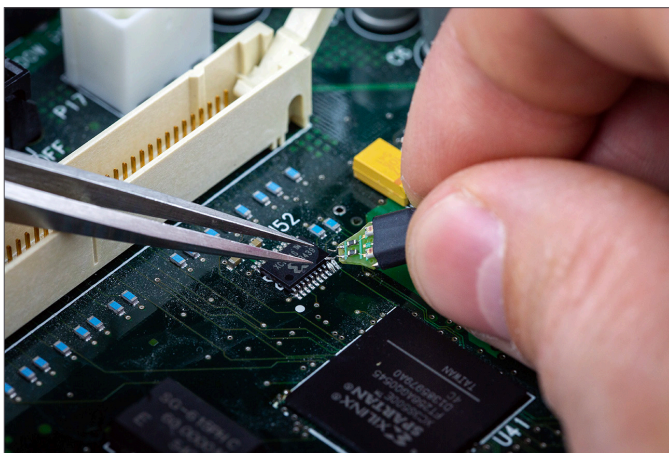
Figure 13: Adjust the tip leads using tweezers if necessary.
