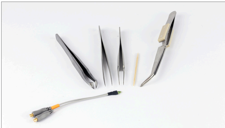
Figure 7: A variety of tweezers is useful for soldering probes. From left to right, cutting tweezers, general purpose tweezers, fine-point tweezers, sharpened toothpick, clamping tweezers.
