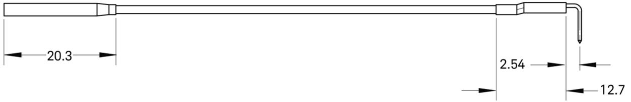
**Figure 7** Ground Lead Dimensions
