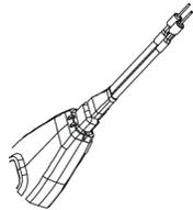
This accessory allows you to extend the reach of the probe with a solder-in probing option.
