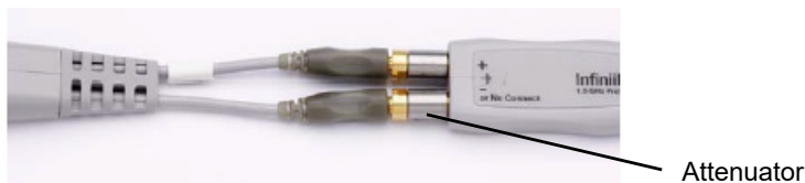
Figure 2 Attenuators Between a Probe Amplifier and a Probe Head
