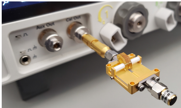
Figure 73 MX0104A deskew fixture connected to oscilloscope's Cal Out connector
