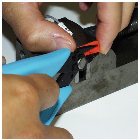
Figure 31 Cutting Wires Flush with Gauge
