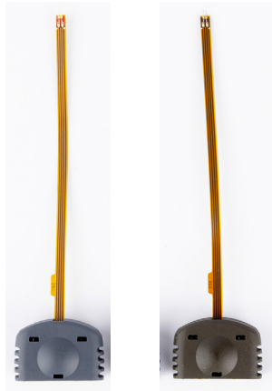
MX0100A Probe Head Before and After Usage under High Temperatures
