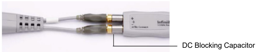
Figure 4 Placement of DC Blocking Capacitor Between a Probe Amplifier and a Probe Head
