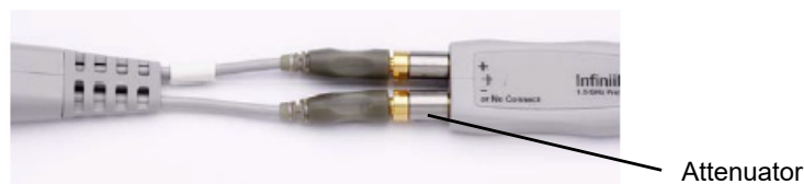
Figure 3 Attenuators Between a Probe Amplifier and a Probe Head
