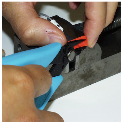
Figure 32 Cutting Wires Flush with Gauge
