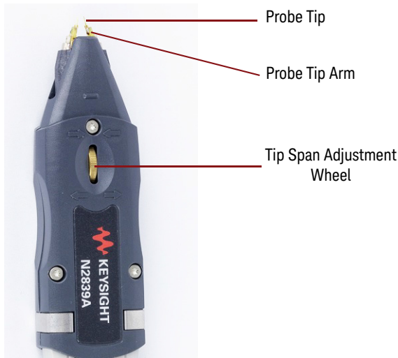
Figure 34 N2839A Browser Probe Head Components
