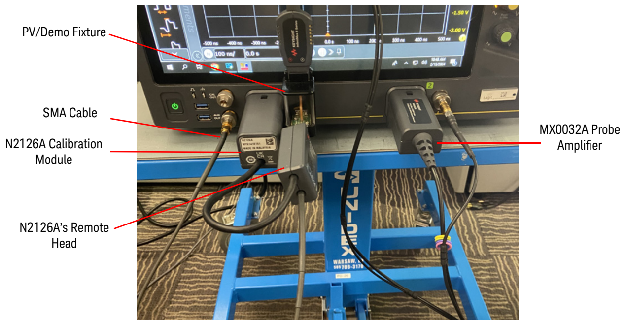
Figure 35 Performance Verification Setup
