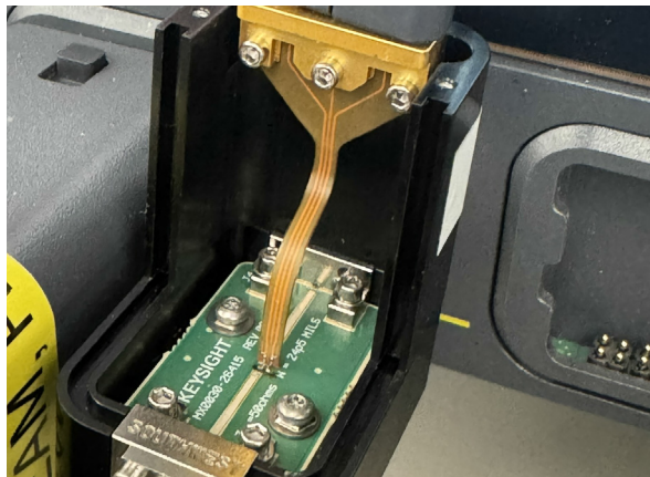
Figure 15 MX0041A probe head connected to DUT
