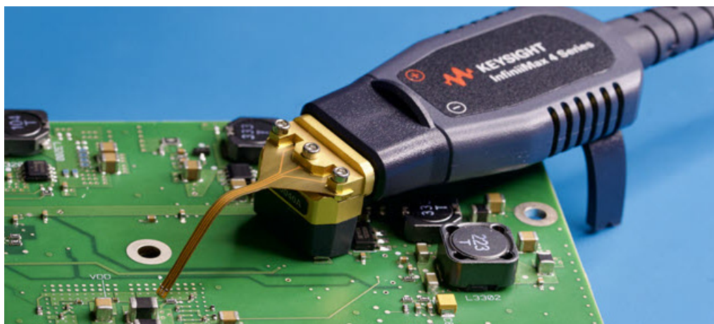
Figure 26 MX0041A probe head connected to probe head connector and horizontal cradle
