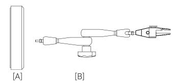
Screw the positioner [B] to the base [A] and tighten it with a combination wrench (width across flats is 7mm).
