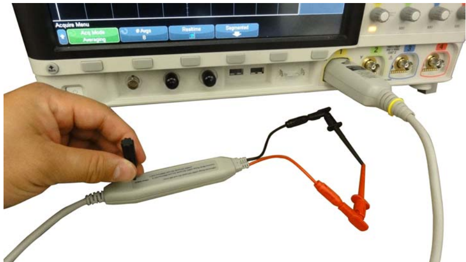
Figure 7 Adjusting the Offset Using the Supplied Tool
