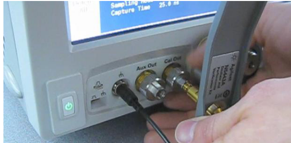
Figure 75 Attaching the N5443A Fixture
