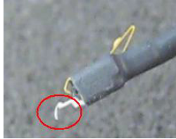
Figure 78 Forming the Probe Head's Tip
