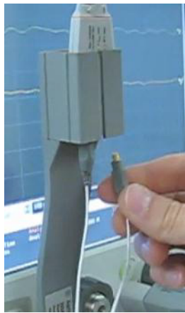
Figure 79 Connect the Head to the Probe
