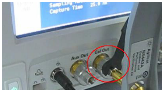
Figure 76 Tighten to 8 in. lbs.
