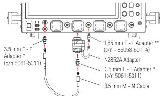
\* 3.5 mm F-F adapter is a standard accessory included with the 1.85 mm / 1 mm UXR oscilloscopes and also with N2852A adapters with a serial number starting with US6127 or higher. N2852A adapters with a serial number less than US6127 are shipped without the 3.5mm F-F adapter.
