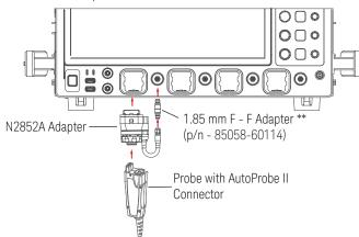
Oscilloscope with 1 mm AutoProbe III Interface Connector
