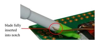
This will keep it from spinning around on the probe while in use. You can also bend and form the blade to reach your grounding location.
