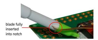
This will keep it from spinning around on the probe while in use. You can also bend and form the blade to reach your grounding location.
