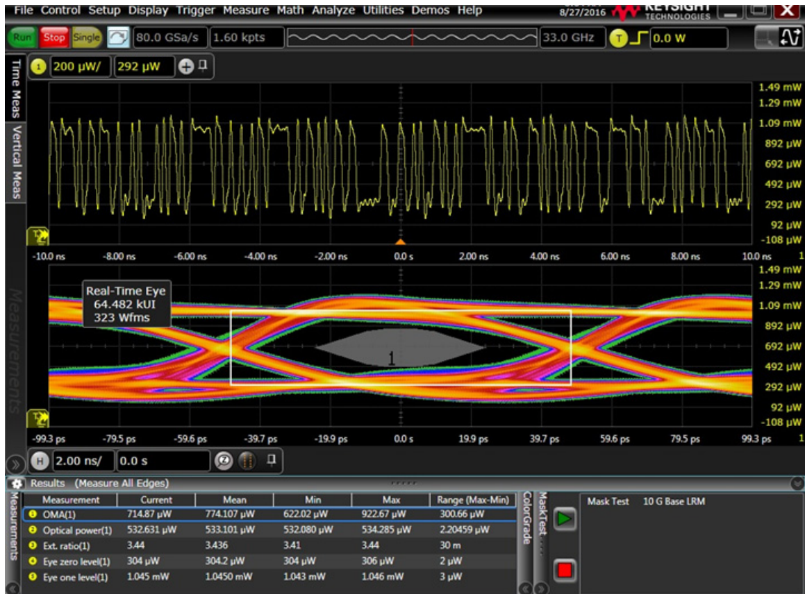
Examples of Optical Data Acquired with N7004A for Different Optical Data Rates For 10 Gbps data rate
