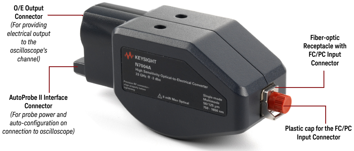
Figure 1 N7004A Optical-to-Electrical Converter - Components
