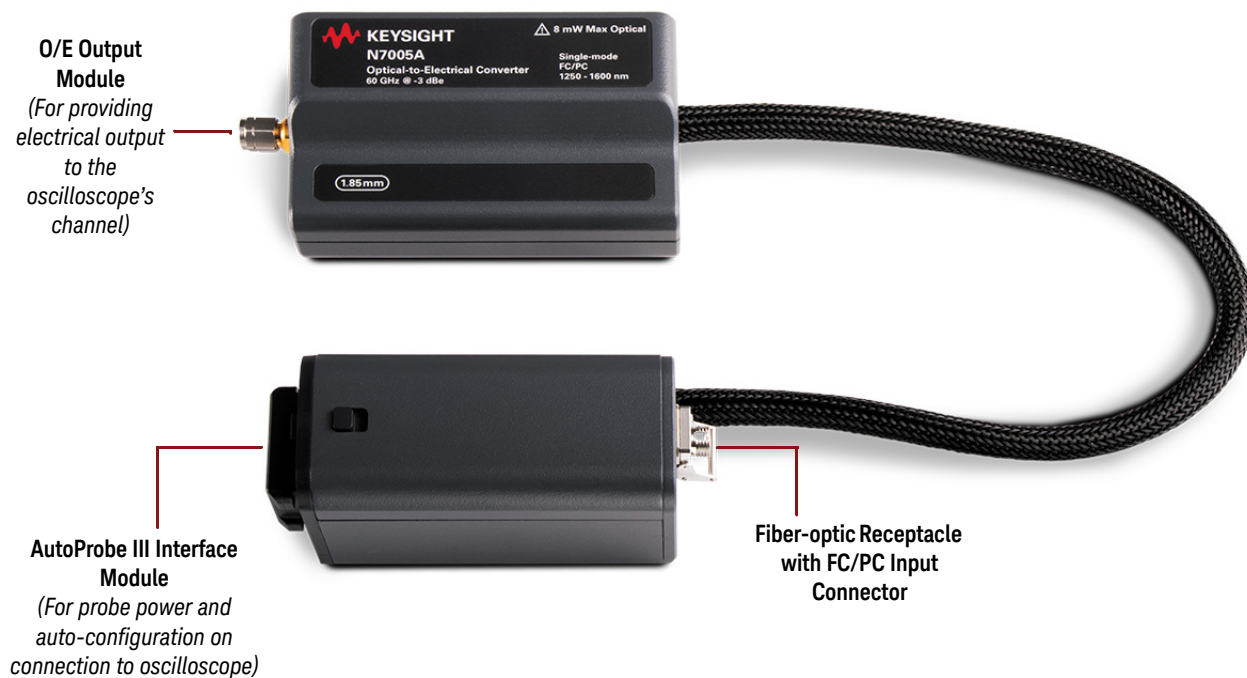
Figure 2 N7005A Optical-to-Electrical Converter - Components
