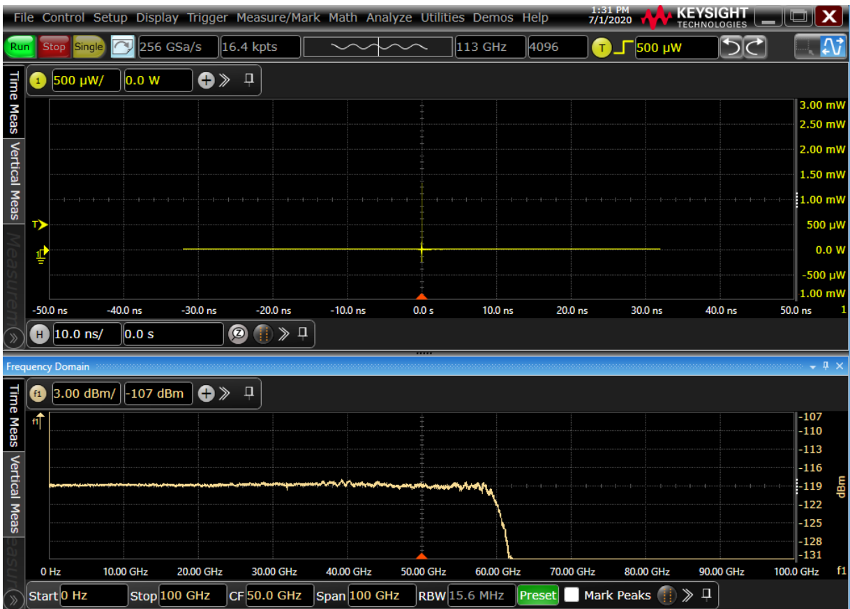
Figure 6 Upper trace: N7005A impulse response. Lower trace: FFT of impulse showing bandwidth
