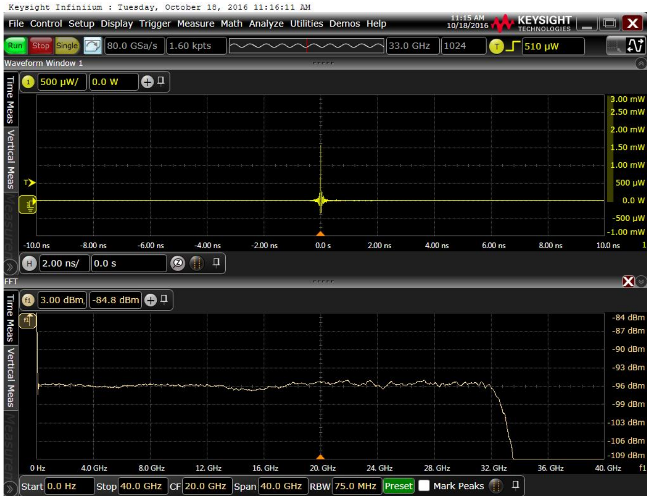
Figure 5 Upper trace: N7004A impulse response. Lower trace: FFT of impulse showing bandwidth
