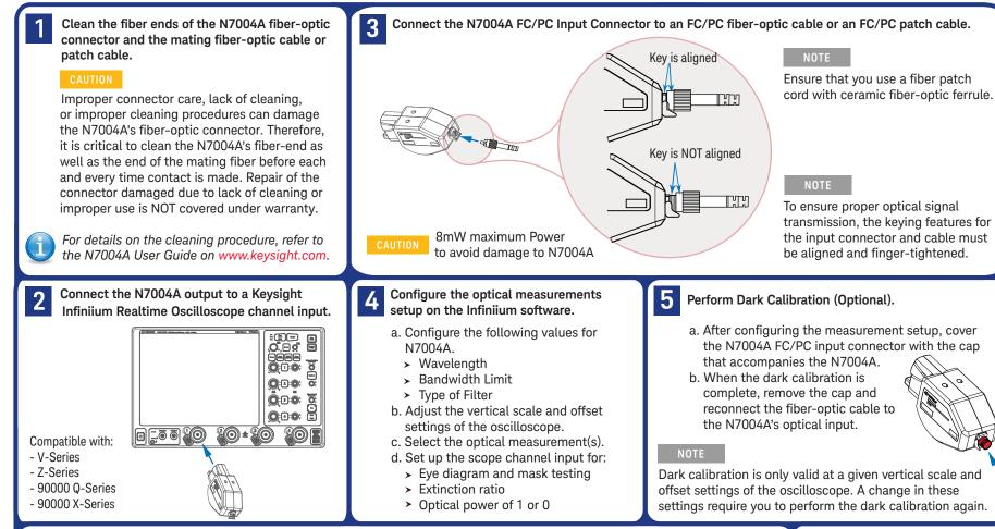
Setup is complete to start making the optical measurements.
