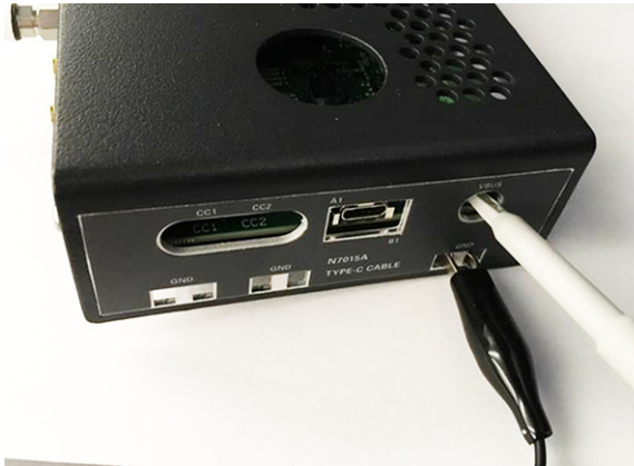
Figure 3 Probing the VBUS at the N7018A
