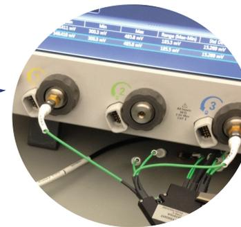
Connect the 2.92 mm connectors of the N7015A fixture to channel 1 and 3 of an Infiniium oscilloscope
