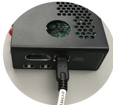
Insert the N7015A Type-C interface cable with the red dot facing up. This ensures proper signal identification.
