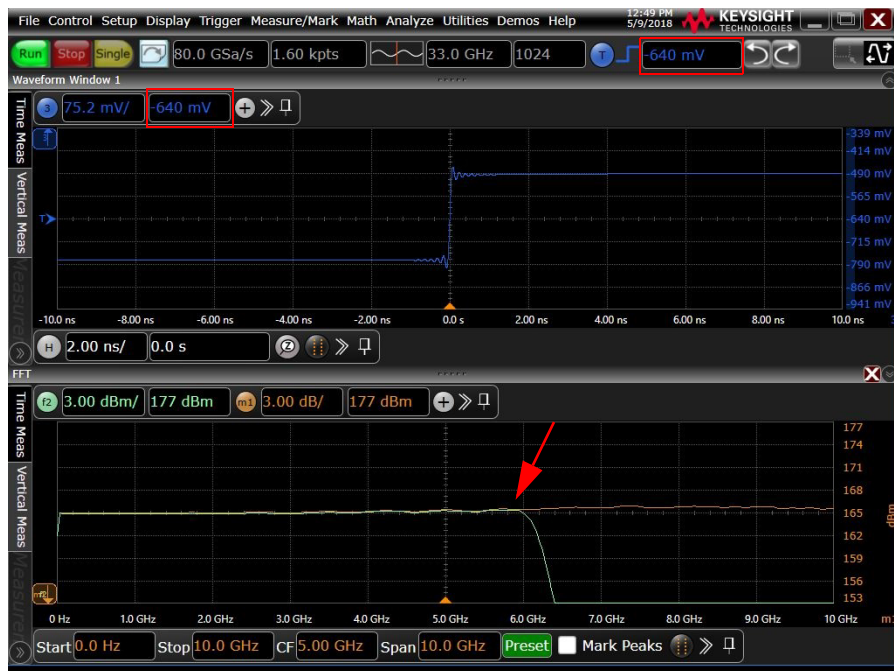
Figure 32 Frequency response of the N7024A probe
