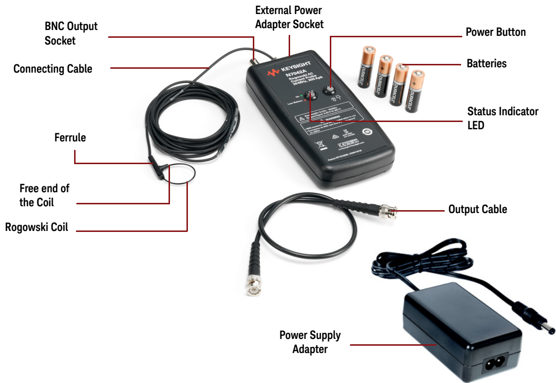
Figure 1 N7040A/1A/2A Probe Components (The figure shows the N7042A probe)
