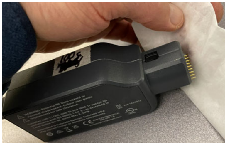
Figure 32 Cleaning probe pogo pins with IPA-saturated wipe
